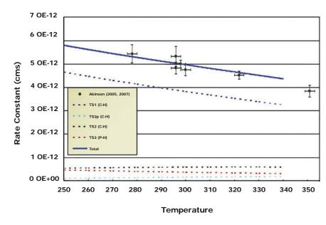
Figure 5. Temperature Dependent Rate Constants for the Reaction of DMHP + OH.
