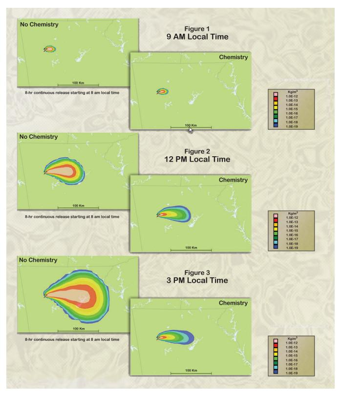
Figure 1. Plume model showing the contamination zone at 9am following the release of 2-methylpropane at 8am.
