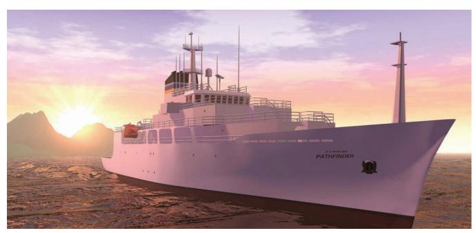
NAVOCEANO has technical control of six 329-foot-long, 5,000-ton T-AGS 60 class ships and one hydrographic ship designed to provide multipurpose oceanographic capabilities in coastal and deep-ocean areas. These include physical, chemical, and biological oceanography; multidiscipline environmental investigations; ocean engineering and marine acoustics; marine geology and geophysics; and bathymetric surveying.
